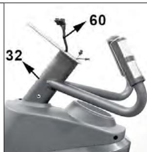
**NOTE:** Guide Upper Connection Wire (60) into Fixed Handlebar (32).
